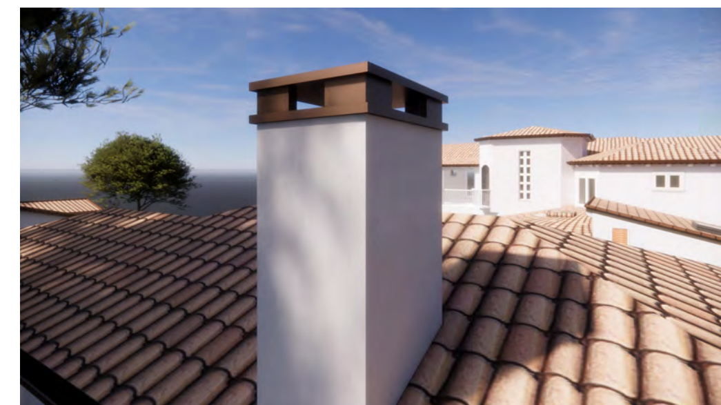
CHIMNEY CAP DESIGN TO MATCH EXISTING (METAL TO BE BRONZE IN COLOR)
