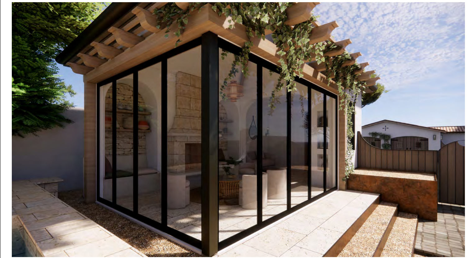
BRONZE METAL FRAME BIFOLDING GLASS DOORS W/ STEEL POST CORNER & EXTRUDED WOOD TRIM
