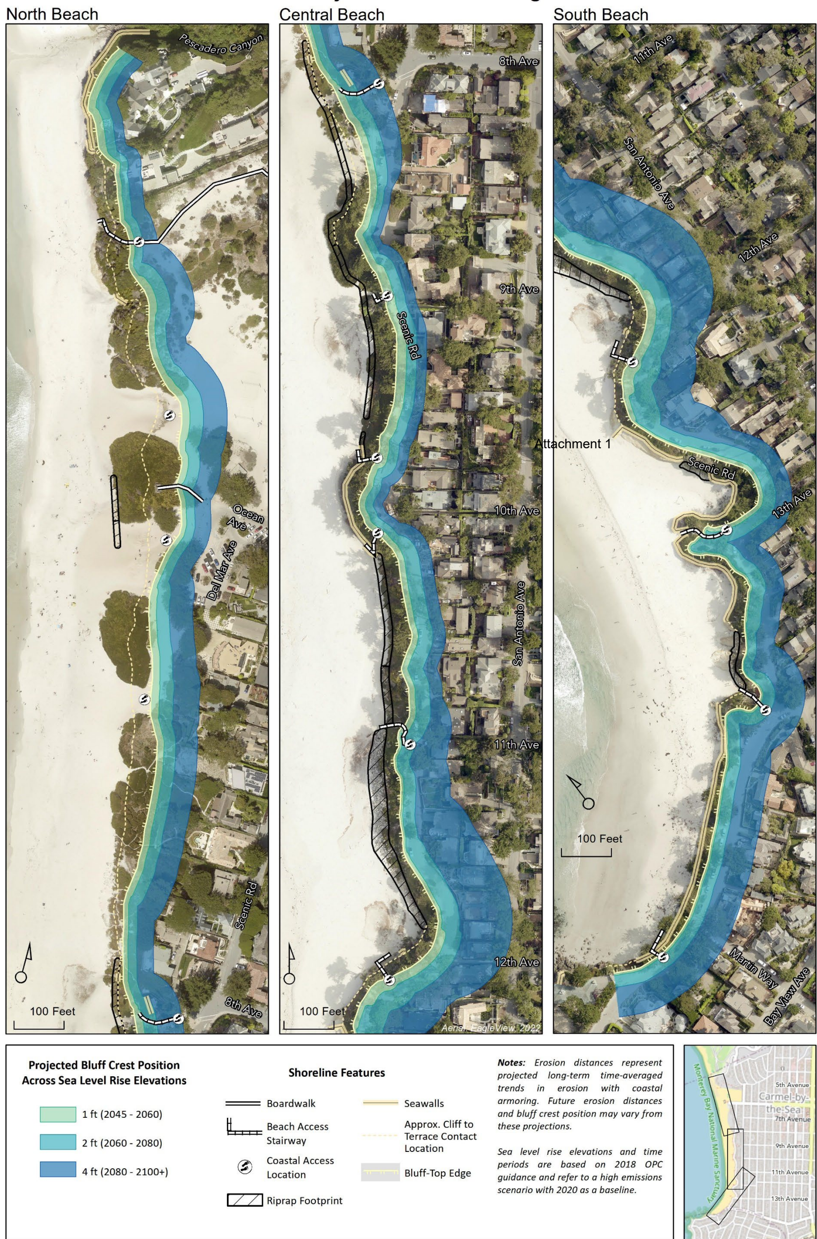
Figure 16. Map of dune and cliff erosion for the entire beach. Displays erosion hazards with armoring. Hazard zones in areas where armoring is not present rely on the ‘without armoring’ scenario using the assumption of an average erosion rate (0.4 ft/yr).
