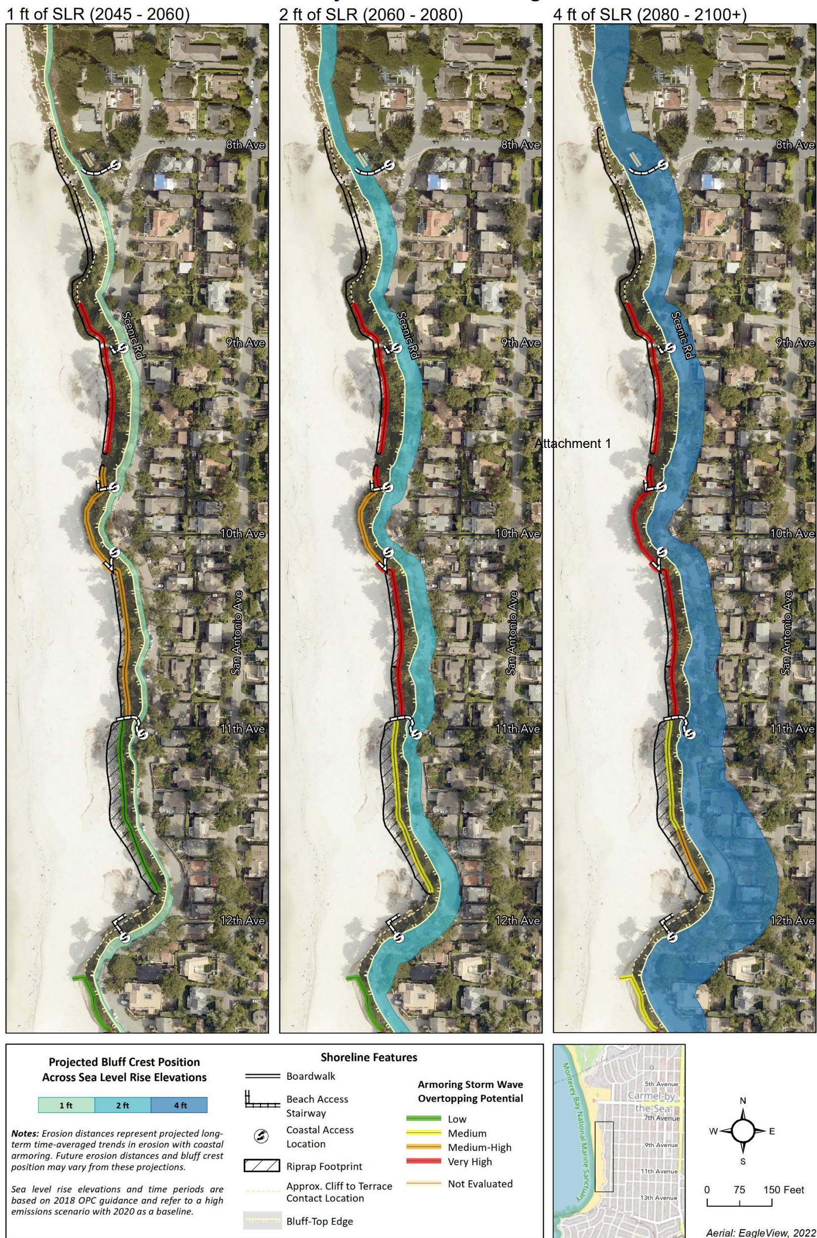
Figure 14. Map of dune and cliff erosion for the central beach. Displays erosion hazards with armoring. Hazard zones in areas where armoring is not present rely on the ‘without armoring’ scenario using the assumption of an average erosion rate (0.4 ft/yr).
