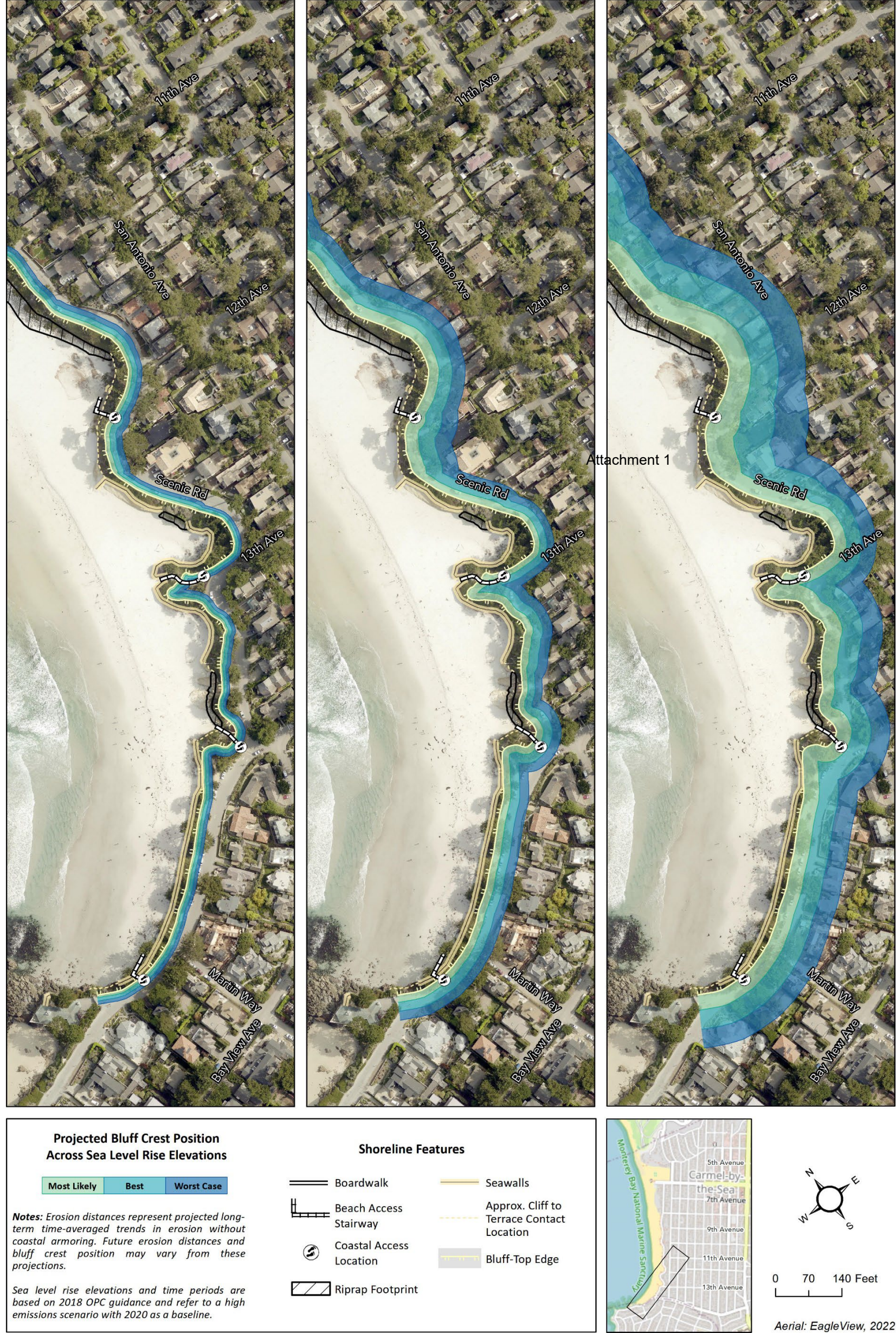
Figure 12. Map of dune and cliff erosion for the southern beach. Displays erosion hazards without armoring. Hazard zones represent three bands of certainty, most likely, based on the assumption of a low average erosion rate (0.2 ft/yr), best, based on the assumption of an average erosion rate (0.4 ft/yr), and worst case, based on the assumption of a high average erosion rate (0.7 ft/yr).
