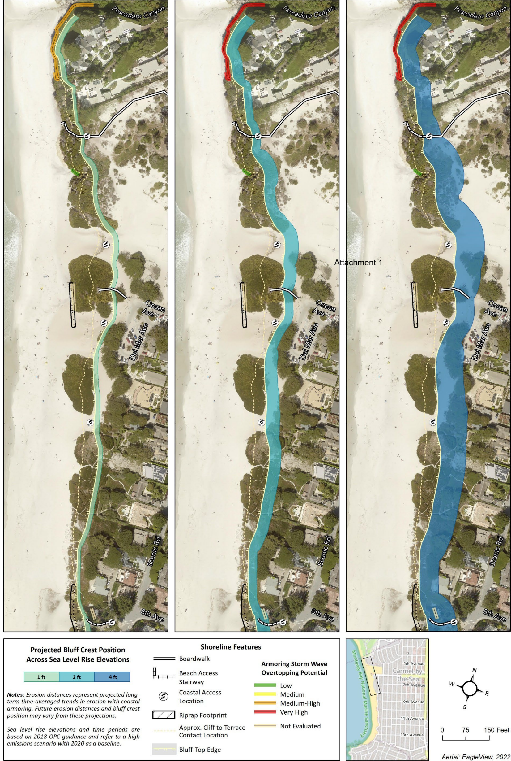
Figure 13. Map of dune and cliff erosion for the northern beach. Displays erosion hazards with armoring. Hazard zones in areas where armoring is not present rely on the ‘without armoring’ scenario using the assumption of an average erosion rate (0.4 ft/yr).
