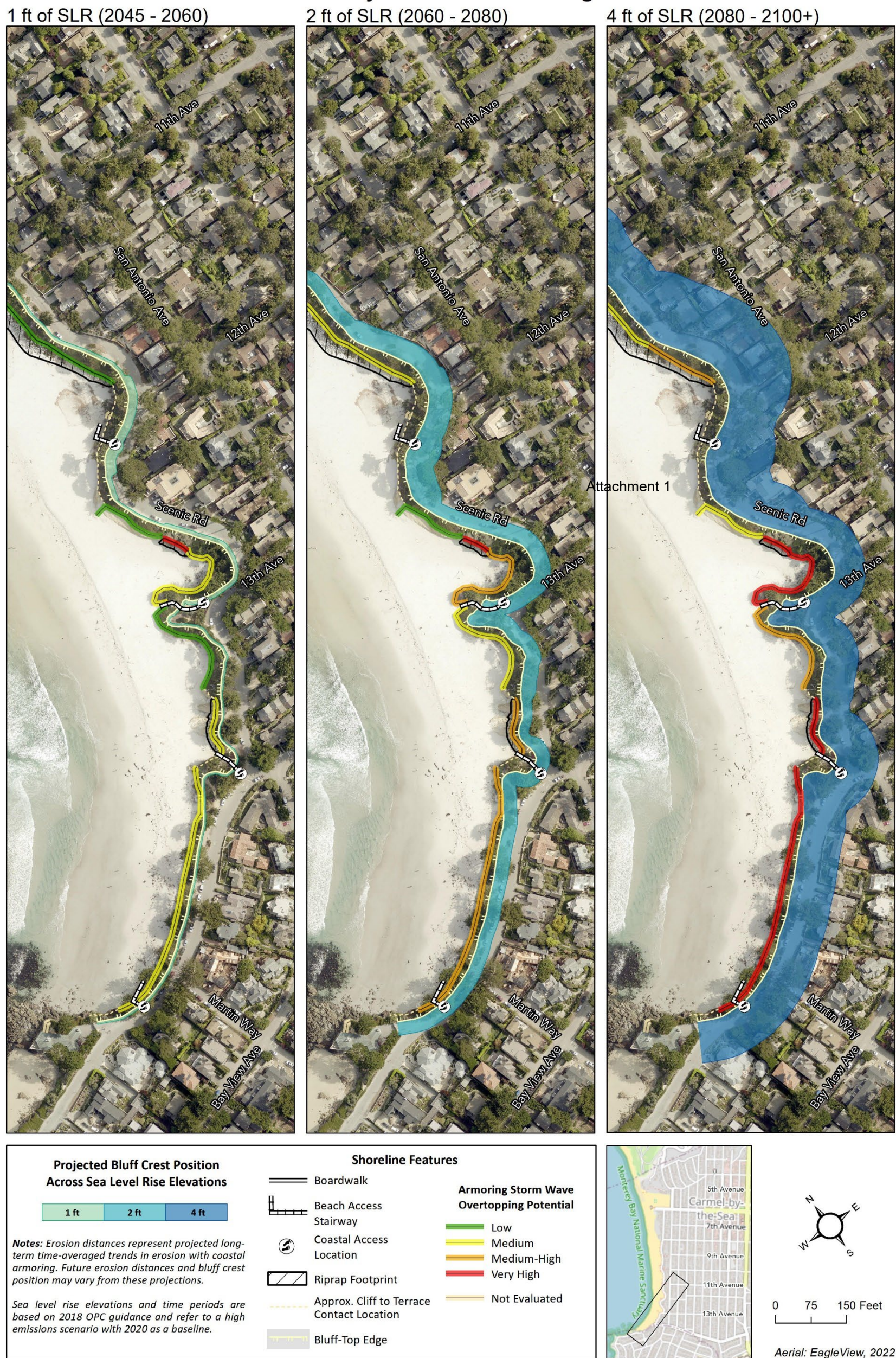
Figure 15. Map of dune and cliff erosion for the southern beach. Displays erosion hazards with armoring. Hazard zones in areas where armoring is not present rely on the 'without armoring' scenario using the assumption of an average erosion rate (0.4 ft/yr).
