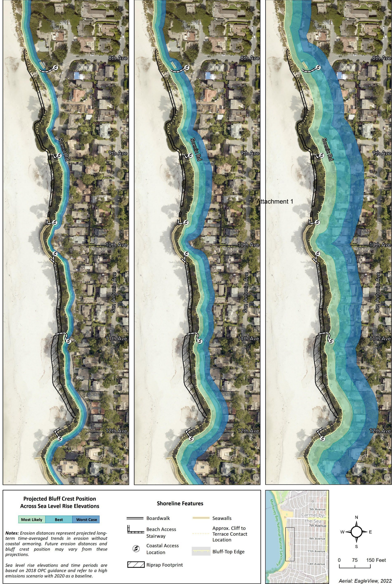
Figure 11. Map of dune and cliff erosion for the central beach. Displays erosion hazards without armoring. Hazard zones represent three bands of certainty, most likely, based on the assumption of a low average erosion rate (0.2 ft/yr), best, based on the assumption of an average erosion rate (0.4 ft/yr), and worst case, based on the assumption of a high average erosion rate (0.7 ft/yr).
