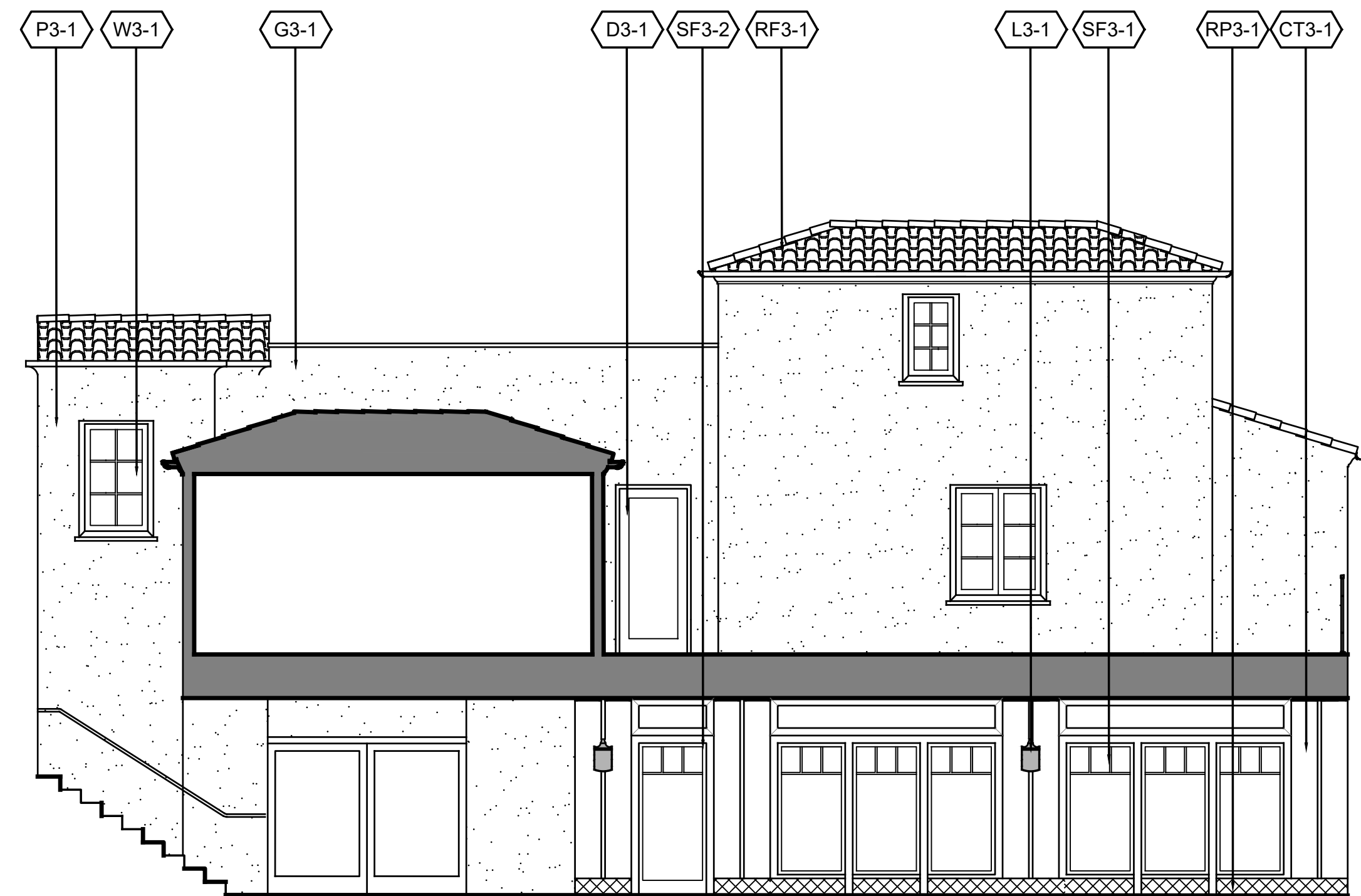
4 BUILDING 3 WEST ELEVATION SCALE: 3/16"=1'-0"
