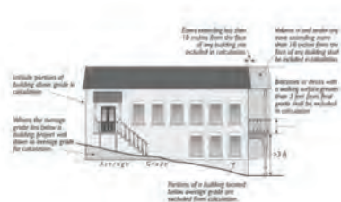
Figure 17-1: Determining Exterior Volume
